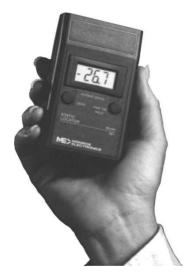
**NOTE** — If, as you approach the target, the indicated field strength begins to exceed 20kV at a distance greater than 1", **STOP!** This implies that the target voltage may be high enough to create an arc. Proceed with caution.
